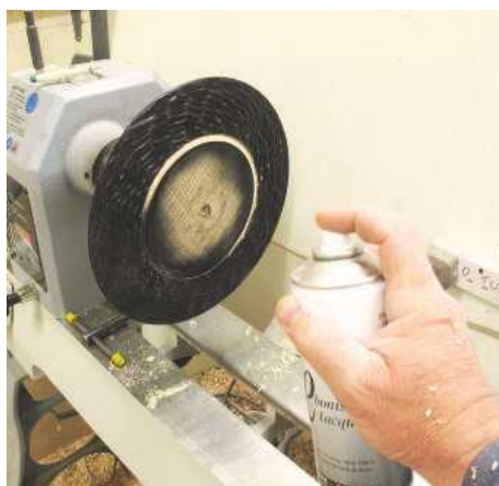
▲ Pic.17 Cut a groove 3mm wide x 3mm deep where you want the texture to end and the bowl to begin. Spray the whole thing, including the groove, black with ebonising lacquer
